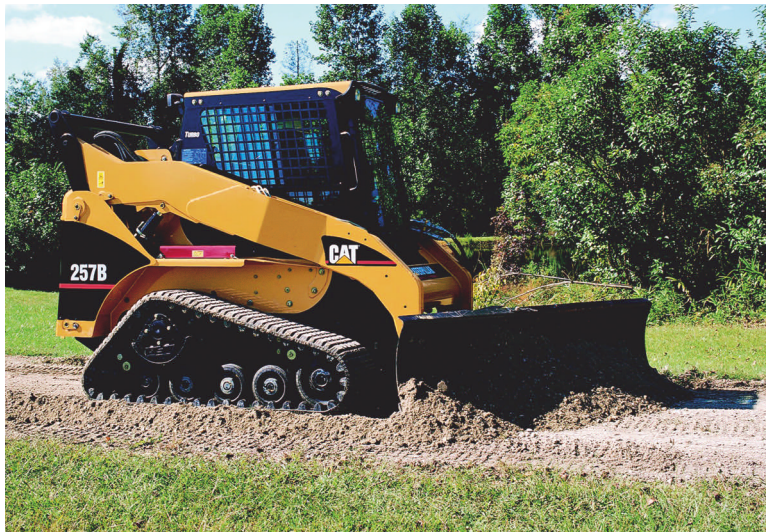
Angle blades are better suited for general earthmoving and snow removal than fine grading. Source: The Cat Rental Store
