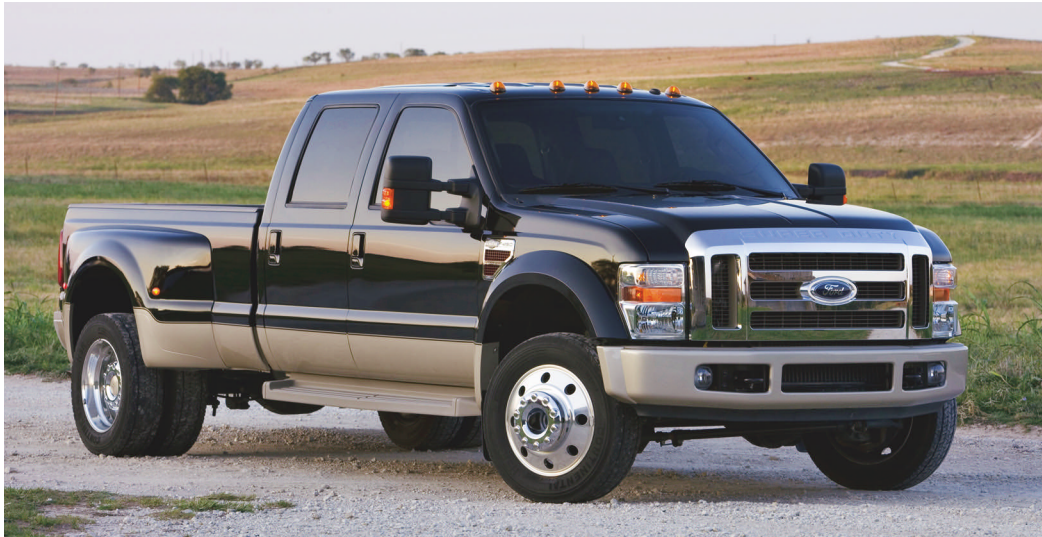
F-450 Pickup combines a versatile hauling bed with a stronger chassis for towing a trailer weighing up to 24,500 pounds. The bed comes in lengths of 6-3/4 or 8 feet.
