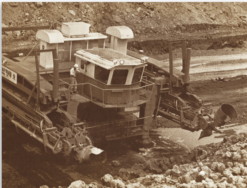
Robbins H-100 horizontal drill was able to simultaneously punch two horizontal holes up to 10-5/8-inch diameter into the overburden.
