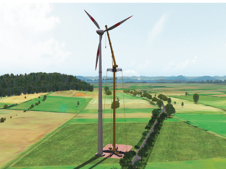
According to Manitowoc, the GTK1100 may have a maximum hook height in excess of 460 feet. Initial testing, says the company, suggests the crane will lift loads exceeding 77 tons to heights exceeding 394 feet.
