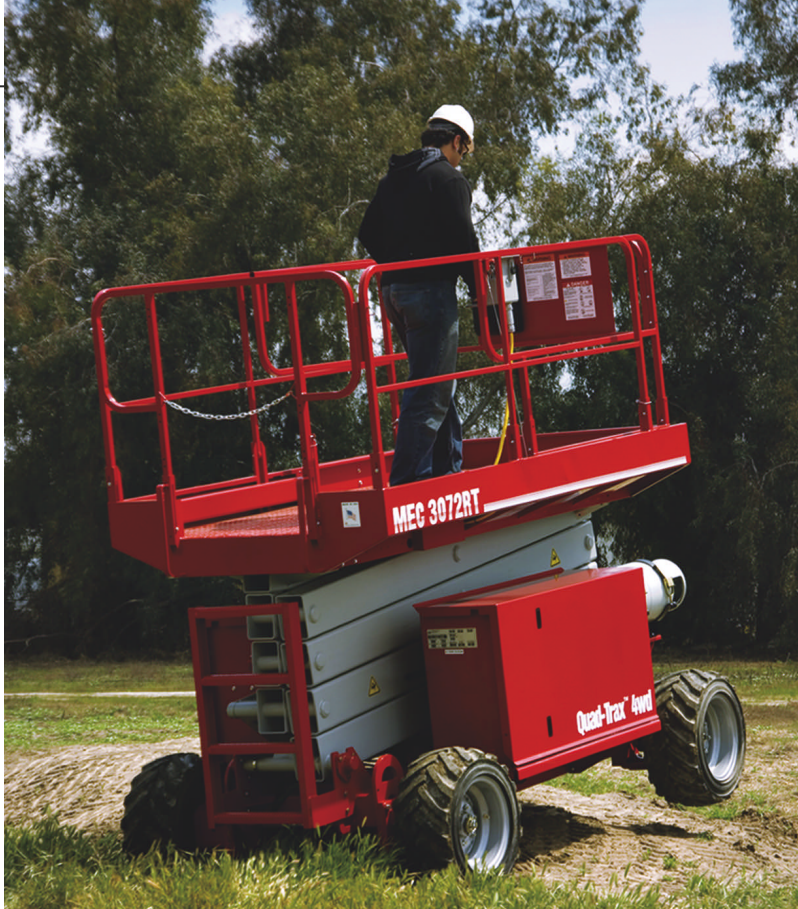
MEC's rough-terrain drive system has three modes, with a Quad-Trax mode that splits oil flow to four separate circuits for all-wheel traction. Each motor senses load, and if one wheel loses contact with the ground, the machines' full power is diverted to the wheels with traction. Model 3072RT can climb 45-percent grades.
