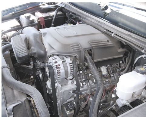
Vortec Max 6-liter V-8 has an aluminum block and various mechanical and electronic advancements. Maybe the neatest is Active Fuel Management, which turns the V-8 into a V-4 when power demand is low.
